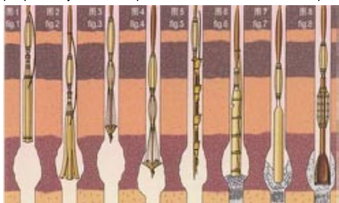
Figure 5. A series of diagrams showing the steps taken to repair a well bore cave in. The first four steps establish the top and bottom depths of the caved in zone; in the fifth step straw is inserted ~ 1m below the zone, where it expands as it soaks up water and plugs the hole; in step six a material is tamped down above the straw to plug the hole more securely; in step seven repair cement (tong oil + lime) is forced into the cave in zone; finally in step 8 a guided bit drills down through the centre of the repaired zone to reopen the well bore.
