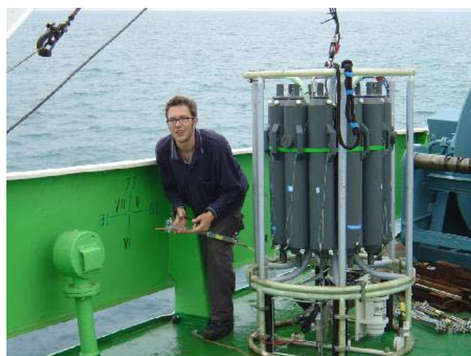
Photo: To obtain the water samples we used a rosette sampler with 12 sampling bottles which could be closed off at different depths by a signal from the ship.
