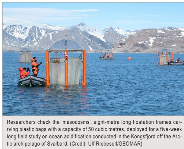
Researchers check the 'mesocosms', eight-metre long floatation frames carrying plastic bags with a capacity of 50 cubic metres, deployed for a five-week long field study on ocean acidification conducted in the Kongsfjord off the Arctic archipelago of Svalbard. (Credit: Ulf Riebesell/GEOMAR)
