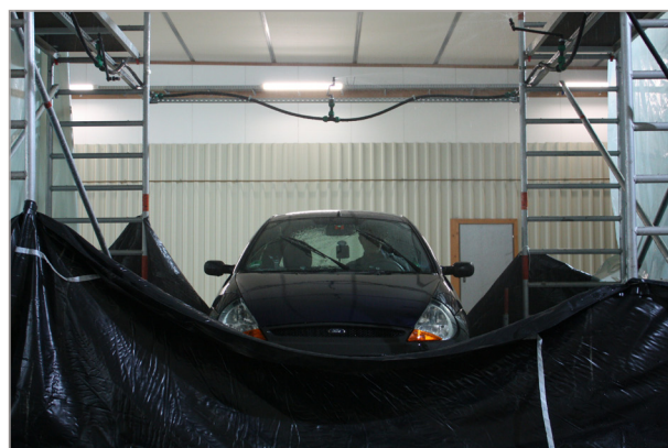
A car tested under a rain simulator. An individual in the car adjusts the wiper speed manually depending on the windscreen visibility. The visibility is related to the intensity of the rain. This is set by the rain simulator, a machine that uses a sprinkler irrigation system with adjustable nozzles to simulate light to heavy rain. (Credit: www.ikg.uni-hannover.de , Daniel Fitzner)
