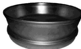
No discard material retained on the 425-μm sieve
