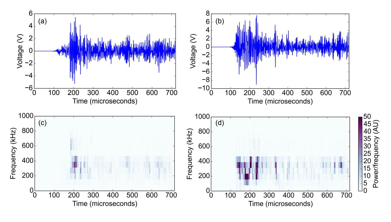
The signals (a), (b) and their corresponding frequency spectograms (c) and (d) show how the first arrivals are recorded with a higher amplitude and broader spectrum when the AE transducer is within the waveguide.
