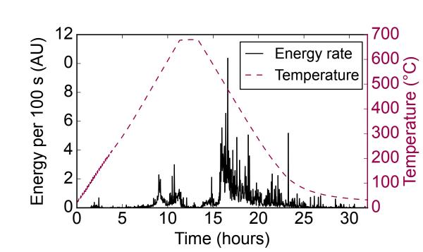
Darley Dale sandstone heated to 700 °C at 1 °C/min and 1 MPa constant uniaxial load (servo-controlled). The hit rate increases with temperature from around 100 °C. The quartz alpha-beta transition (~573 °C) sees an increase in the hit rate. Most of the recorded acoustic energy is released during heating.
