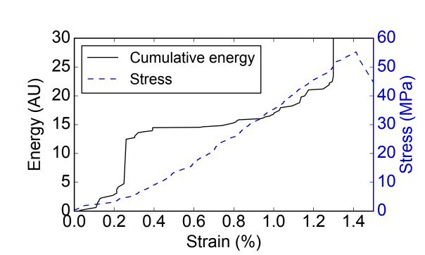
These graphs show the results of AE monitoring of a uniaxial test at room temperature on Darley Dale sandstone and are presented to underline the wide spectrum of possible tests combining mechanical and thermal stress with this setup.
