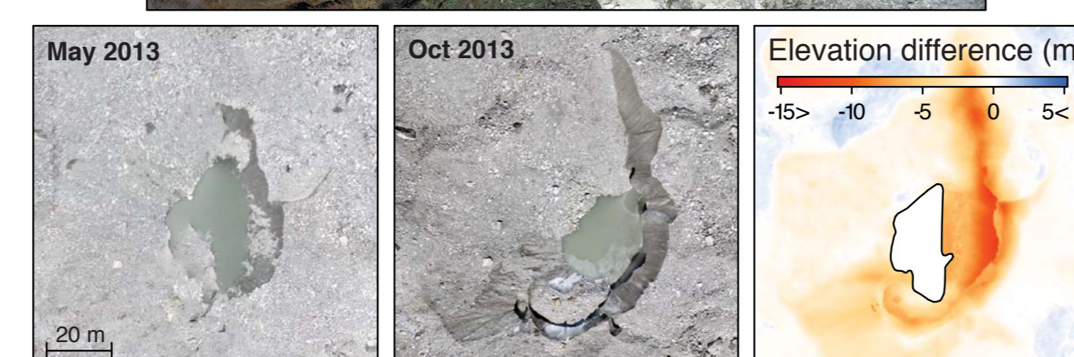
Figure: Heterogeneous patterns of elevation change observed over the 2013 monsoon season. Ice cliffs found on Lirung are highly dynamic and have considerable influence on total melt. Elevation gains in the bend because of emergence.
