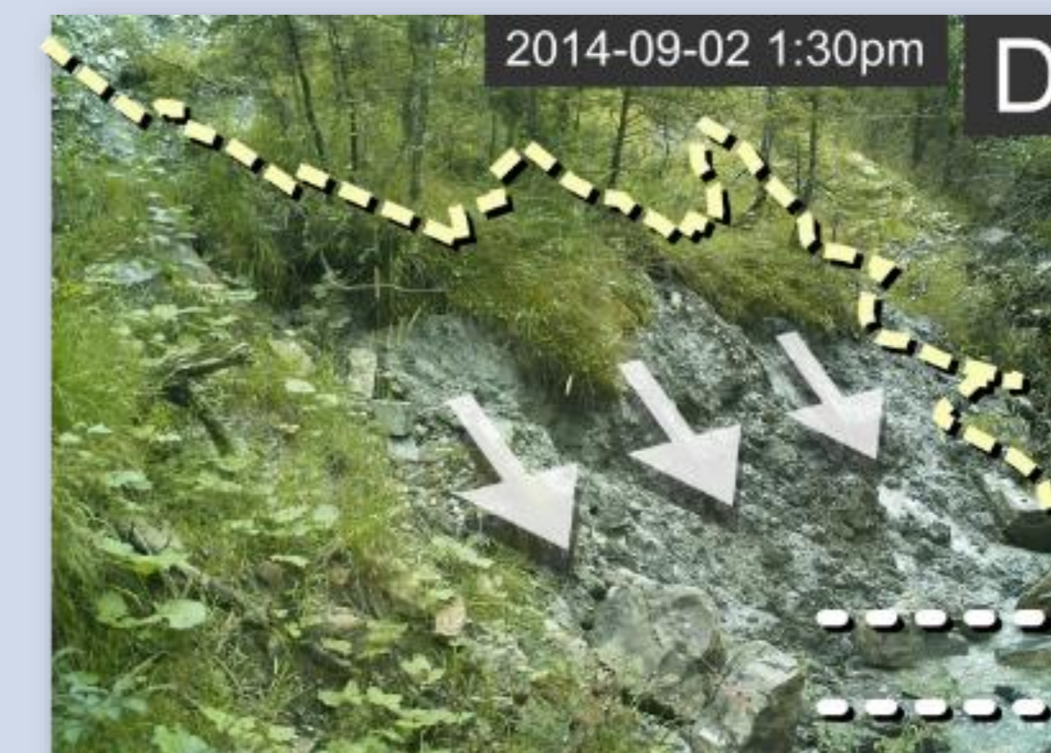
Fig. 3D: 40 hours after peak discharge, the landslide entered a 45 day phase of continuous integral motion (Fig. 4), during which precipitation averaged 10.8 mm/d.
