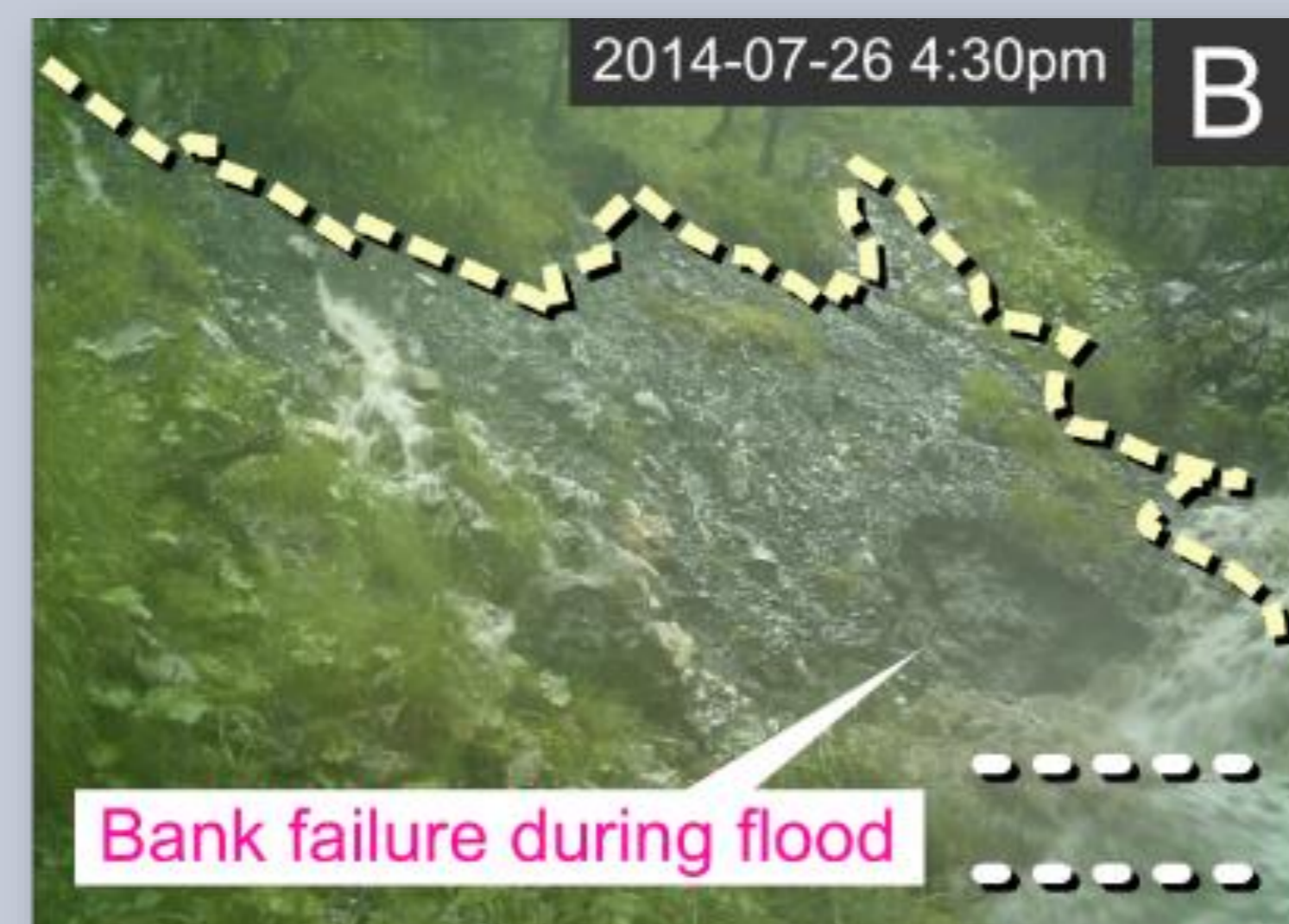
Fig. 3B: A flood on 26 July with a 5-year return period. Although the magnitude of the discharge of this event was the highest on record, rainfall during previous events was higher (Fig. 5).
