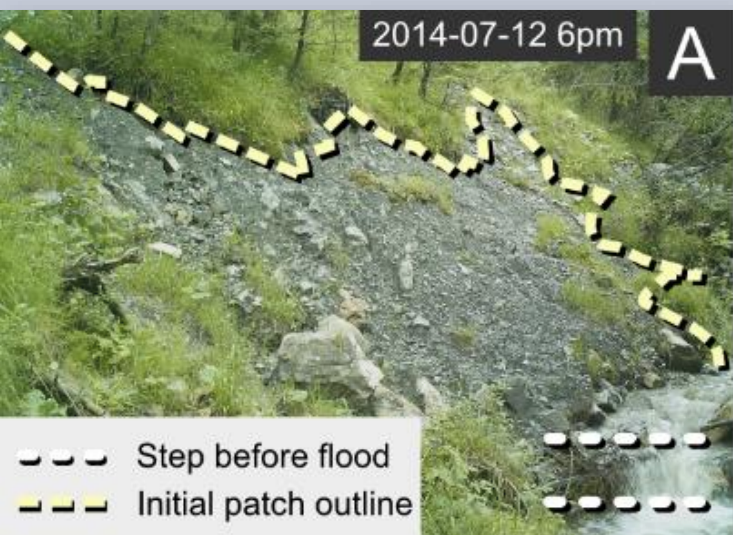
Fig. 3A: The hillslope before 26 July 2014. It shows no measurable surface displacement for several months (Fig. 4), despite 55 precipitation events totaling 1073 mm of rain (10.1 mm/d on average).
