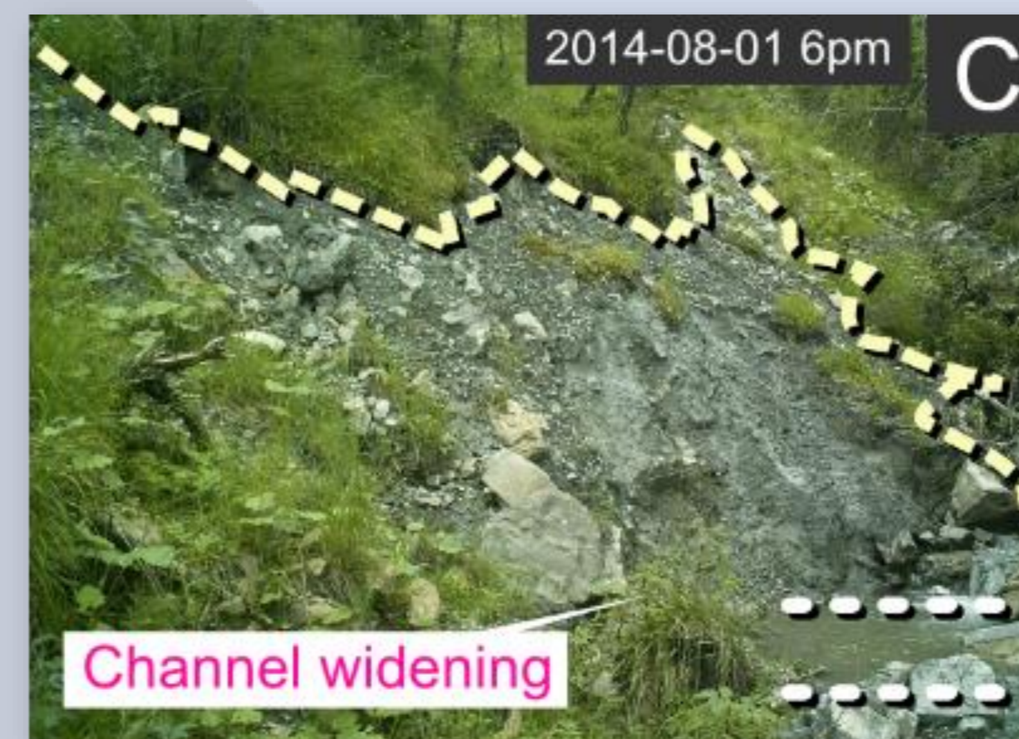
Fig. 3C: While previous events had not noticeably modified the monitored reach, this flood resulted in an ~4 m upstream migration of the alluvial step at the downstream end of the landslide.
