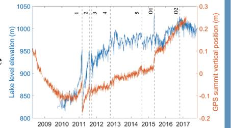
Fig.6: Lava lake level and GPS summit vertical elevation (proxy for inflation and pressurization of magma chamber) over time. 1-ERZ eruptive event (Kamoamo eruption), 2-ERZ eruptive, 3-ERZ eruptive, 4-ERZ intrusive, 5-ERZ intrusive [6], O1-O2 for overflows
