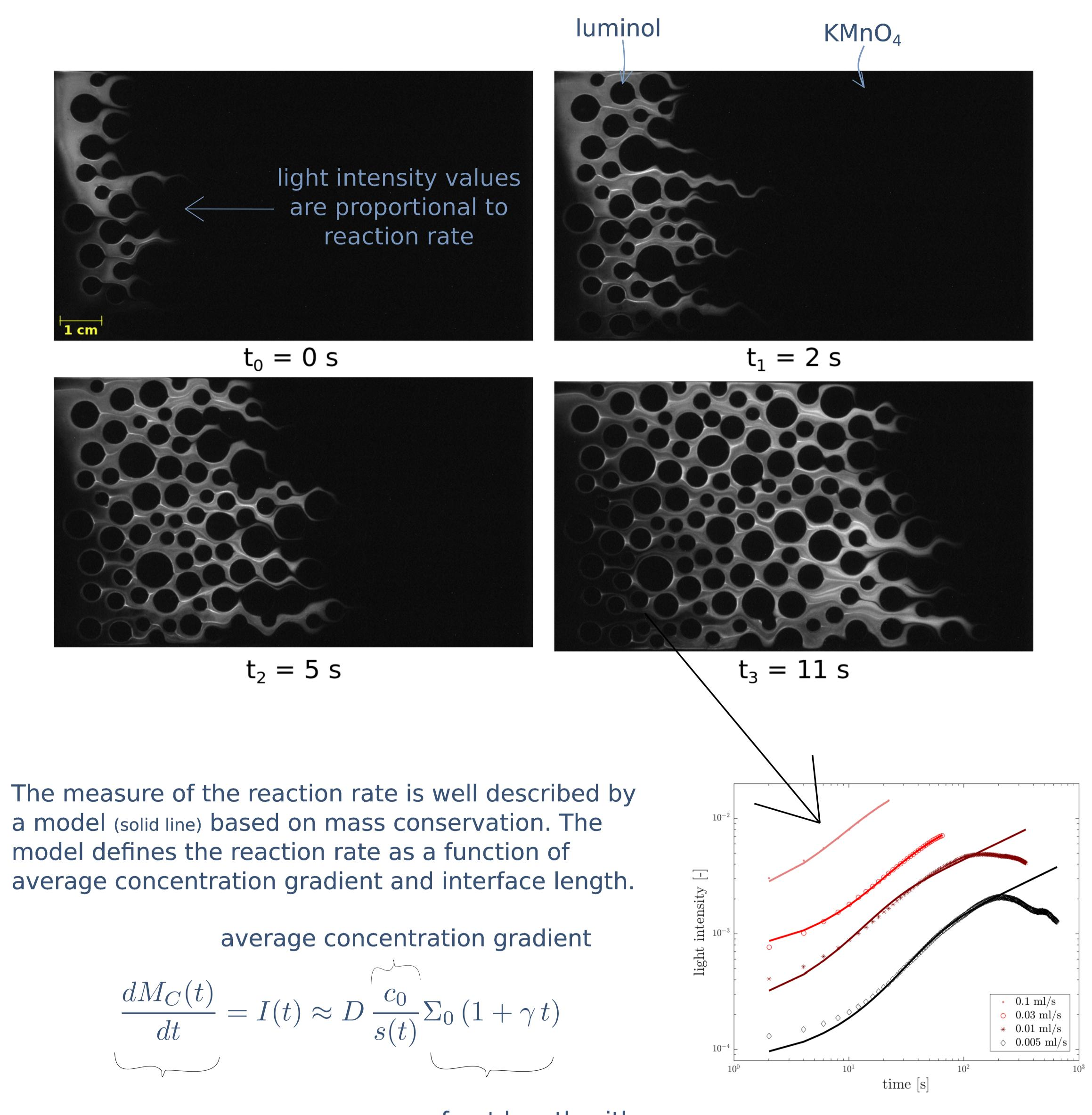
Time evolution of mass of product C, measured by the light intensity of the reaction between solutes A and B. front length with stretching rate  $\gamma$  measured during the conservative experiment
