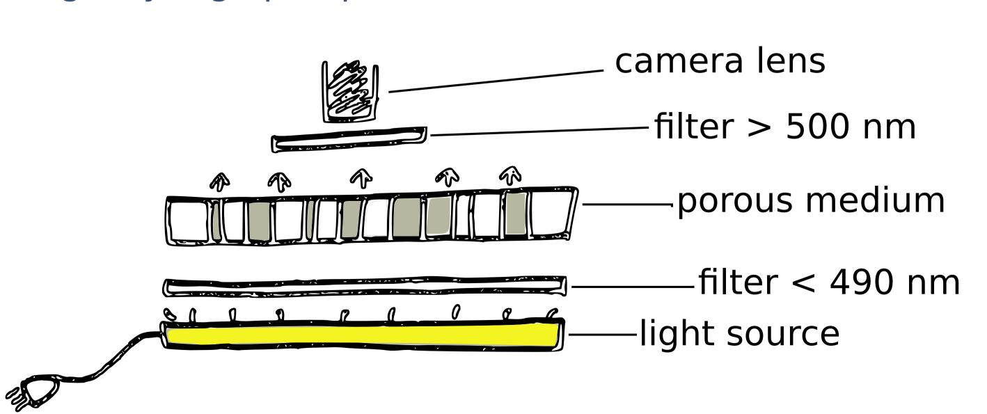
Fluorescein is used as conservative tracer; the fluorescent tracer is excited by a light source at a wave length of 494 nm and emits back at 512 nm, a pair of low-pass and band-pass filters allows that only the signal emitted by the tracer reaches the camera lens.
