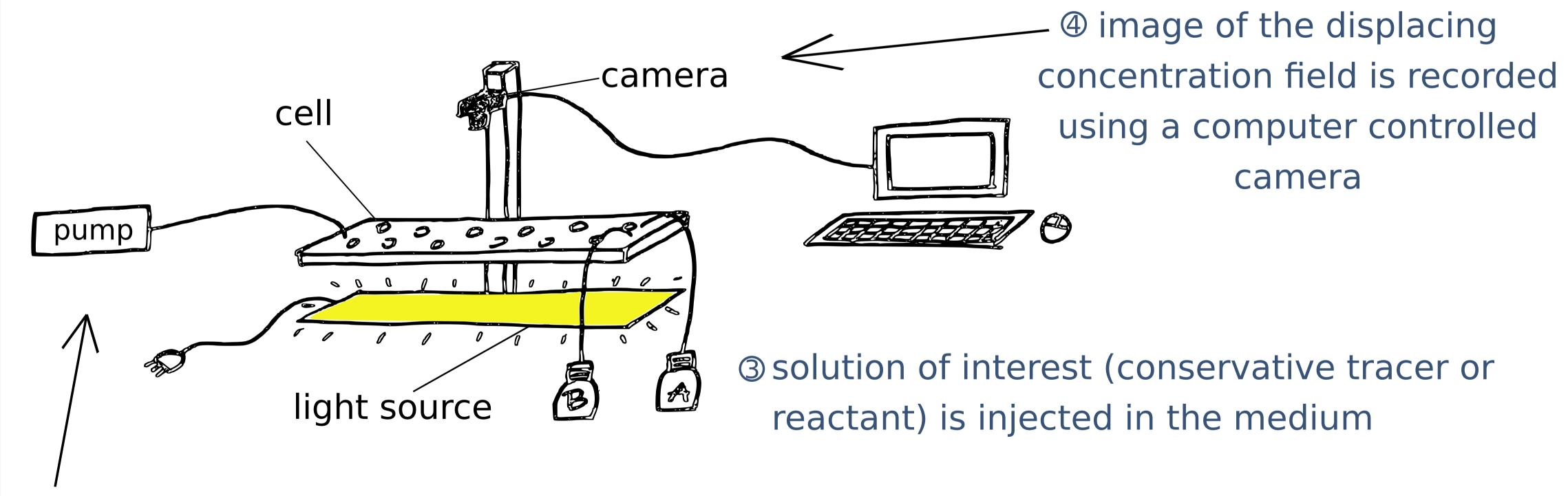
Oflow is created using a syringe pump
