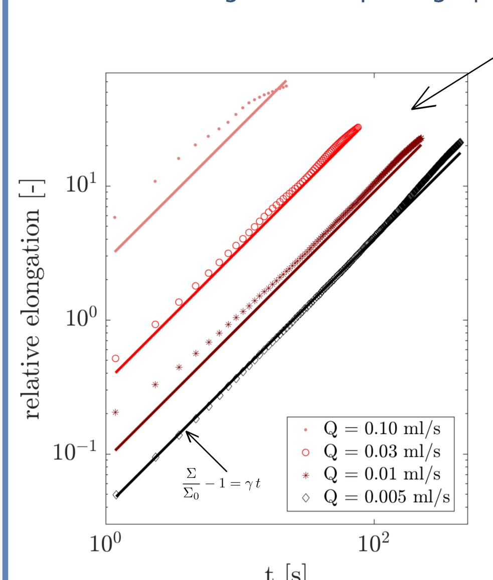
Time evolution of the measured interface between tracer and resident water for different flow rates. As the concentration field moves forward the heterogeneous structure of the medium stretches the interface in the local flow direction, this results in increasing the length of the interface.
