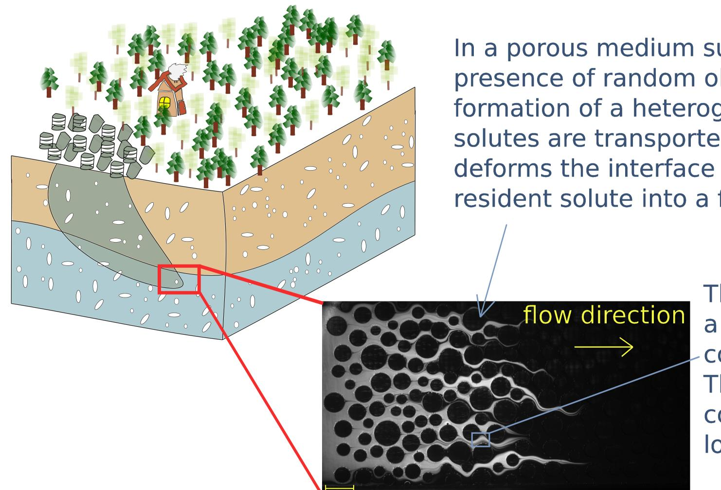
In a porous medium such as a portion of soil the presence of random obstacles (grains) leads to the formation of a heterogeneous flow field. While solutes are transported the contrast of velocities deforms the interface between invading and resident solute into a fingering topography.
