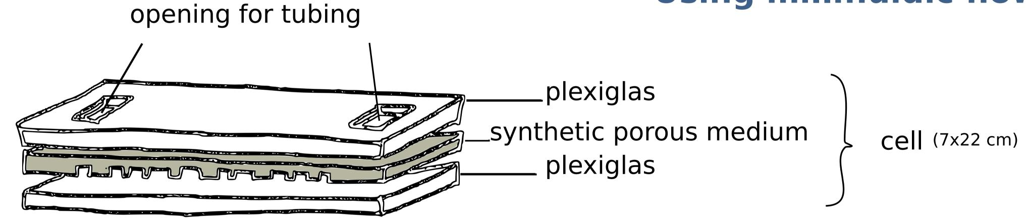
1) porous medium is enclosed between two plexiglas plates and saturated
