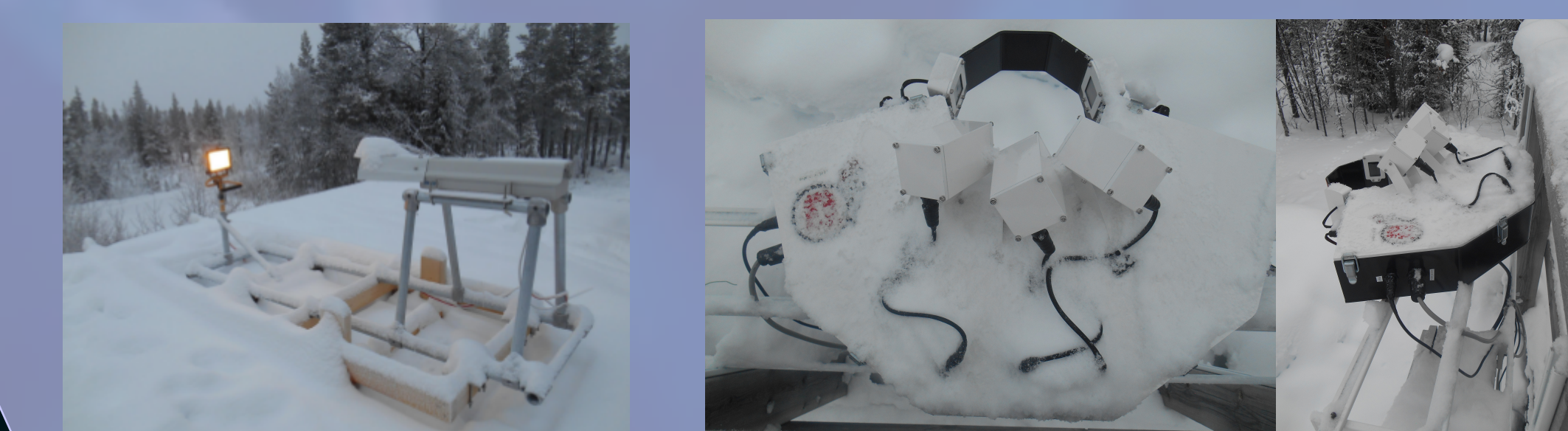
FIG.10: Other ground-based in-situ instruments currently located in Kiruna. Left: PIP (Particle Imaging Package) instrument. Right: MASC (Multi-Angle Snowflake camera) instrument. One photo shows the instrument as viewed from above and the other one from the side.
