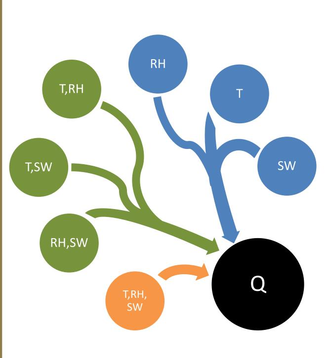
Compute process networks for all combinations of effect of temperature (**T**), relative humidity (**RH**), and shortwave (SW) to turbulent heat fluxes (**Q**) using conditional mutual information (**I(X;Y|Z)**) to understand process interconnections
