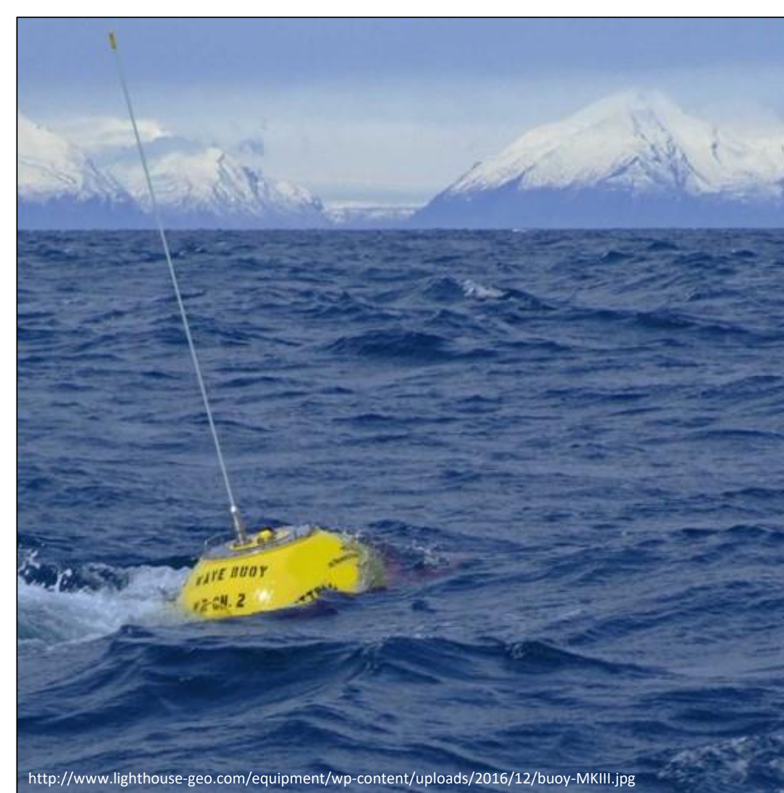
The waverider buoy Mk III is fixed to the seafloor by chains and a rubber band, allowing the floating body to follow the sea surface. Measurement frequency: 1.28 Hz.
