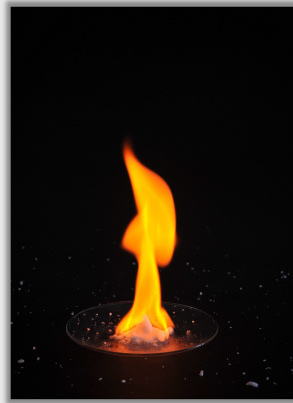
Fig. 1 Burning of methane hydrate sample in the lab
