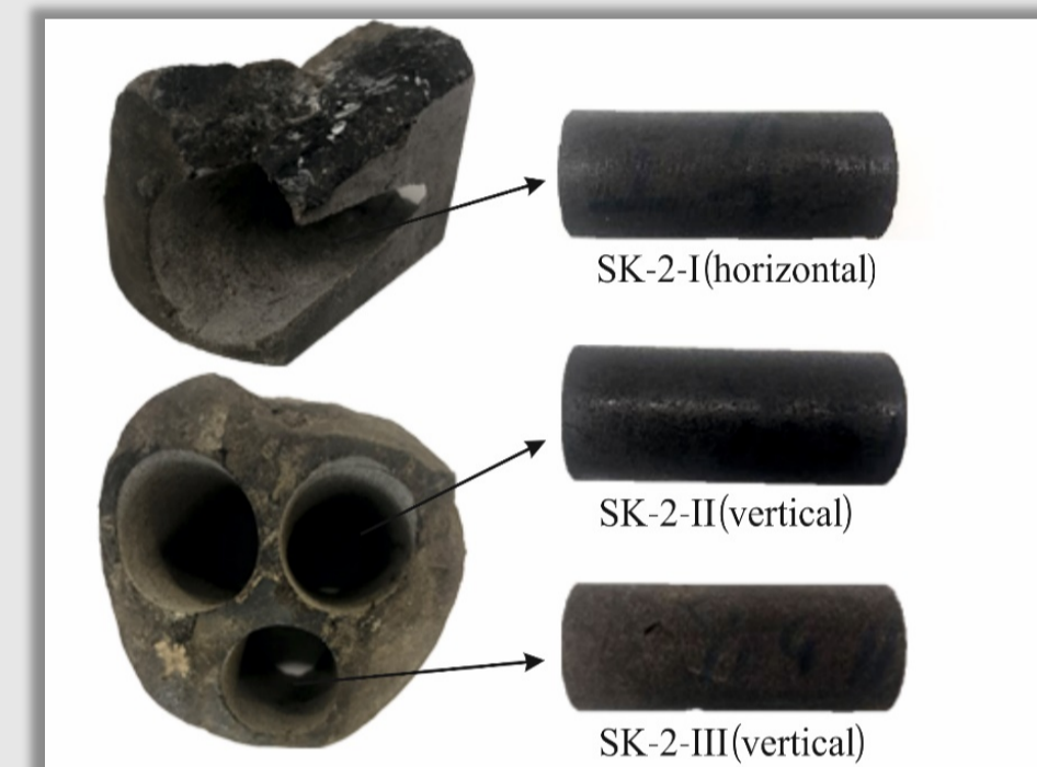
Fig. 4 Samples SK-2-I-III taken from one core piece recovered from borehole SK-2
