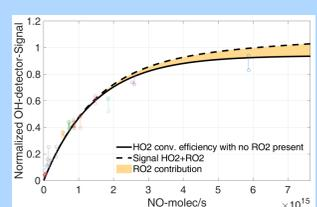
Fig 2d: HO<sub>2</sub> conversion efficiency for different NO additions
