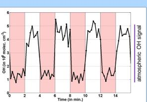
Fig 2b: Determination of chemical background by periodic scavenger addition
