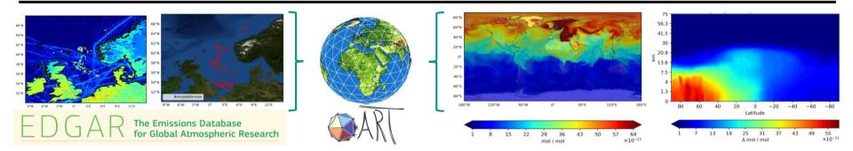
Emission fluxes from the EDGAR inventory are used as input for the global model ICON-ART. North Sea platforms are implemented as point sources. In this way we can adjust missing platform emissions and evaluate their impact on regional and global scale.
