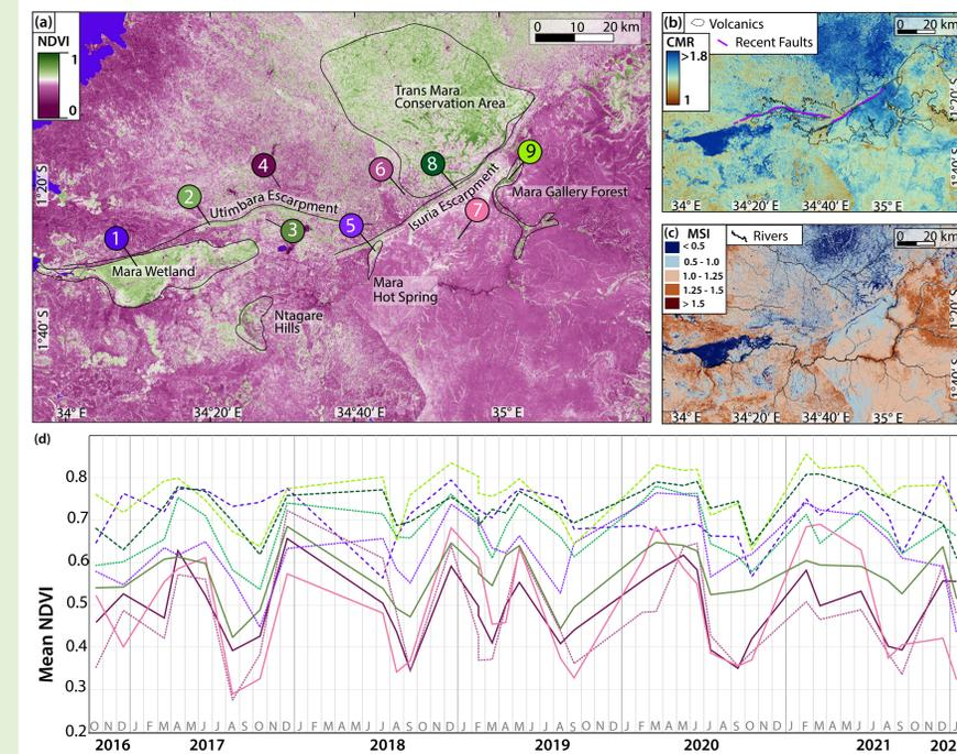
Figure 6 (a) Mean NDVI (b) Mean CMR (c) Mean MSI (d) Temporal distribution of NDVI along the fault zone using a 5-year time series.
