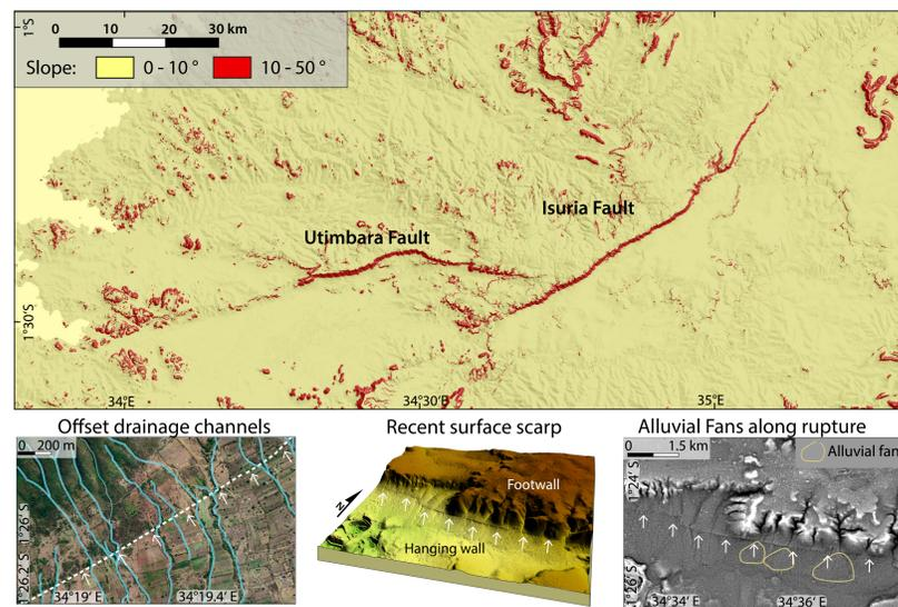
Figure 4 Evidence for fault activity along the Isuria-Utimbara Fault Zone from TanDEM-X [5] and Google Earth imagery.
