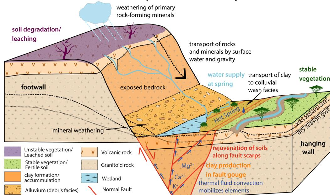
Figure 1 Conceptual model of tectonic activity influencing hydrological and clay forming and/or accumulating processes in a normal fault zone and schematic distribution of different rock types in the study area.
