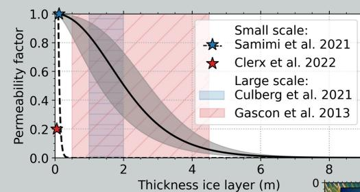
We use ice layer thickness to estimate the permeability of ice slabs to calculate the 'reachable' firn air content (FAC). This method is informed by observational studies.
