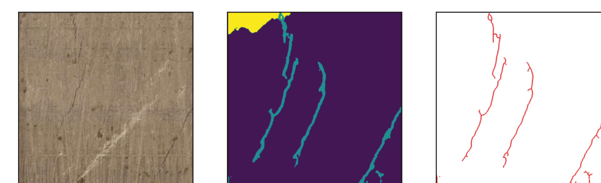
Fig 8. Skeletonize of the prediction. The left one is the original image. The middle one is the prediction from our model. The right one is the skeleton of induced cracks.
