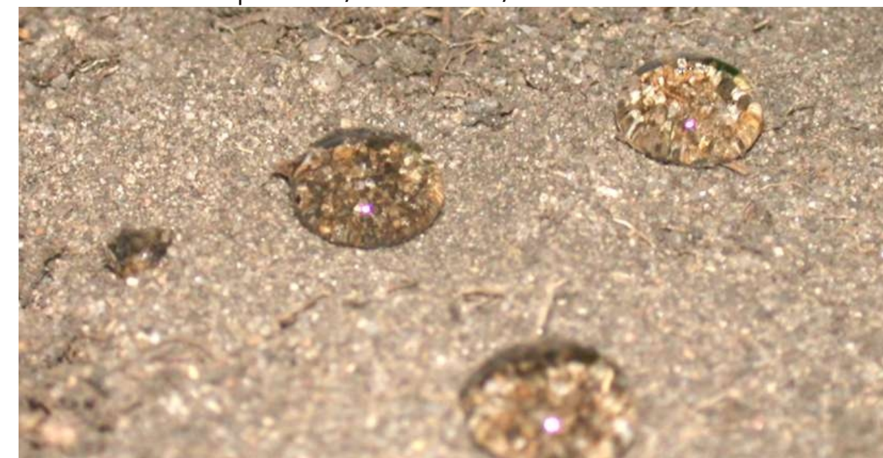
Fig. 2: WDPT test on a water repellent soil sample
