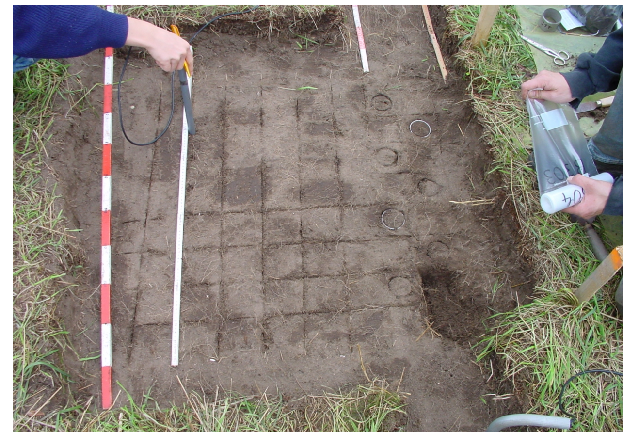
Fig. 1: horizontal sampling in a 10x10 cm grid, visible soil moisture pattern, Oct 2001, Berlin Buch
