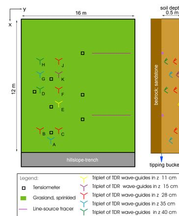
**Fig. 3:** Setup of TDR Triplets at hillslope. *left:* top down view; *right:* profil
