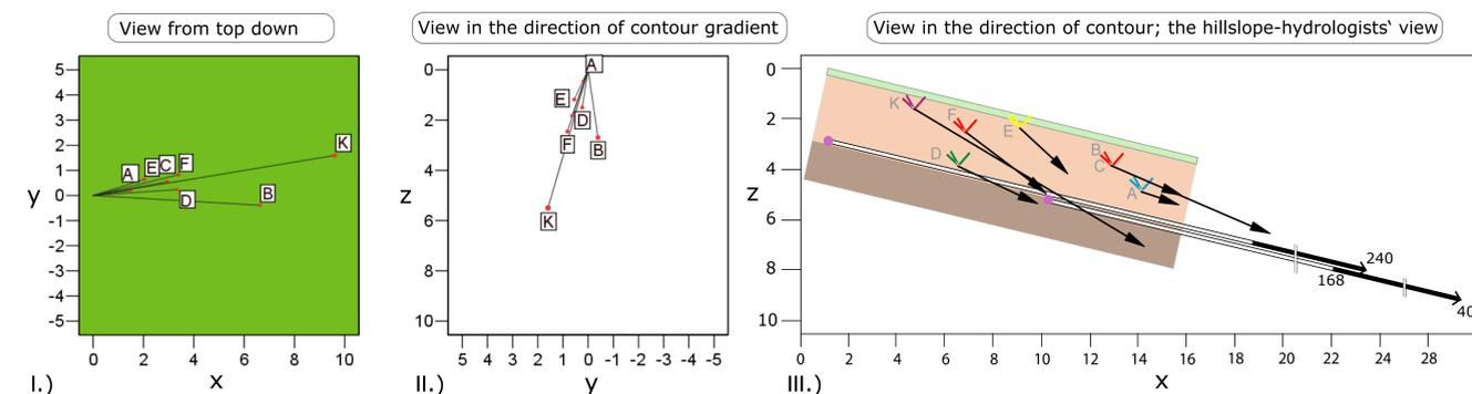
**Fig. 4:** Resulting velocity vectors of the wetting front at various triplets in the hillslope. Unit:  $\text{mm min}^{-1}$ . In III.) additionally velocity vectors ( $\rightarrow$ ) of subsurface storm flow are referring to the line source tracer experiment (first arrival). White subdivision within arrow shows velocity corresponding to peak of mass transport.
