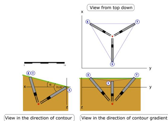
**Fig. 2:** Scheme of mounting three pairs of TDR wave-guides in a hillslope soil.
