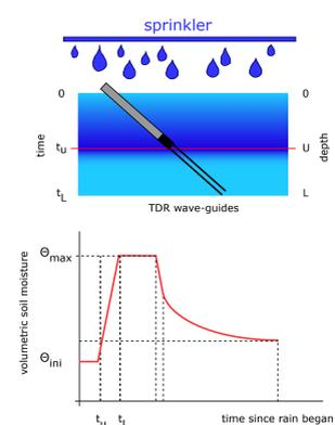
**Fig. 1:** Schematic representation and the linear increase of  $\theta$  as the wetting front moves steadily.
