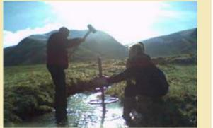
Figure 5: Installation of hyporheic water sampling equipment
