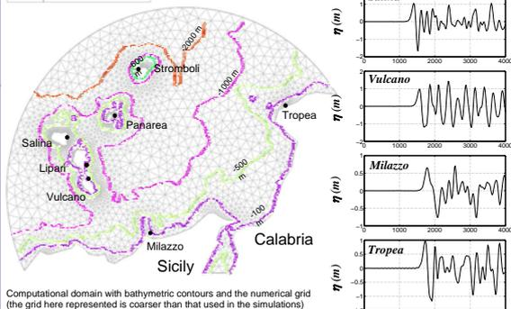
Computational domain with bathymetric contours and the numerical grid (the grid here represented is coarser than that used in the simulations)
