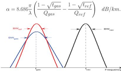
Example of a resonance measured with gas, reference gas, and vacuum conditions
