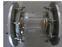
Glass pressure vessel enclosing the resonator
