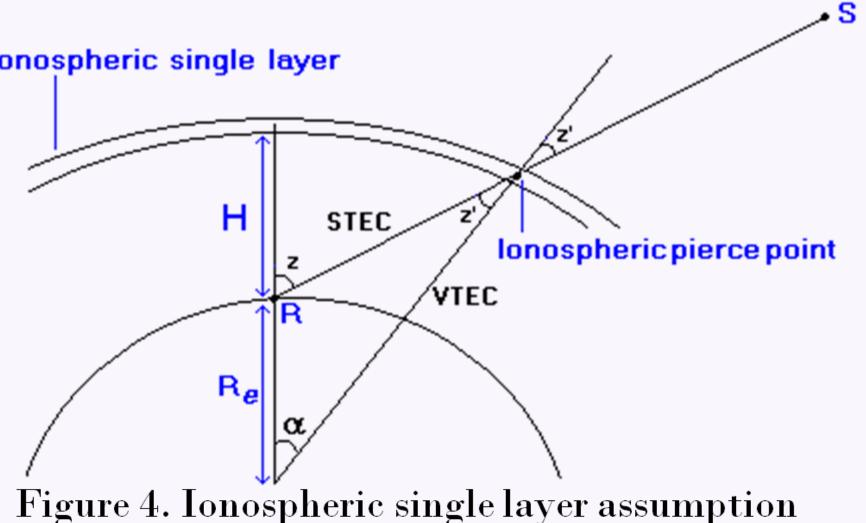
• Ion3 depends on the shape parameter,  $\eta$ , and the maximum electron density in the ionosphere,  $N_{max}$ , that is assumed to occur in a single layer (at height H=450km) pierced at the IPP by the satellite -receiver link (Fig. 4).
