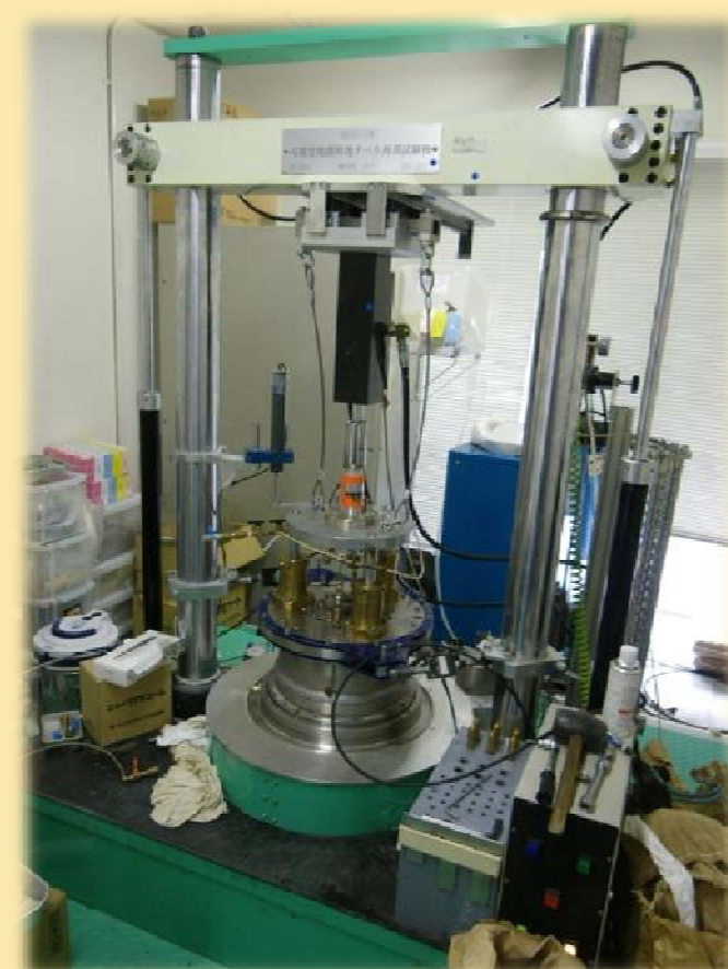
View of the ring shear apparatus DPRI-7 (by Sassa, Fukuoka & their colleagues at DPRI, Kyoto University to simulate the potential landslide sliding surface under earthquakes and rainstorm condition)
