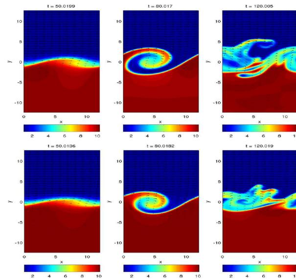
Fig. 3. Time series of the density for  $\rho_1=10$ ,  $k_x a=0.52$ , and  $g=0$  (upper plot) and  $g=12 \cdot 10^{-3}$  (lower plot).
