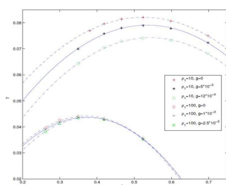
Fig. 1. Normalized growth rate as a function of the normalized wave number for  $\rho_1=10$  and for  $\rho_1=100$  for different values of  $g$ .
