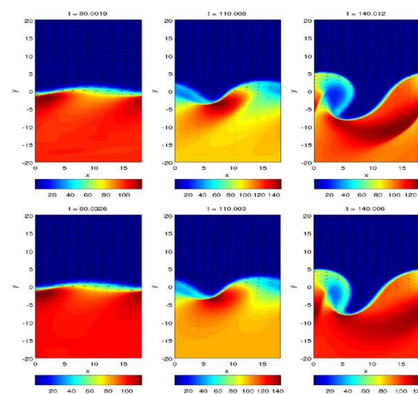
Fig. 4. Time series of the density for  $\rho_1=100$ ,  $k_x a=0.35$ , and  $g=0$  (upper plot) and  $g=25 \cdot 10^{-4}$  (lower plot).
