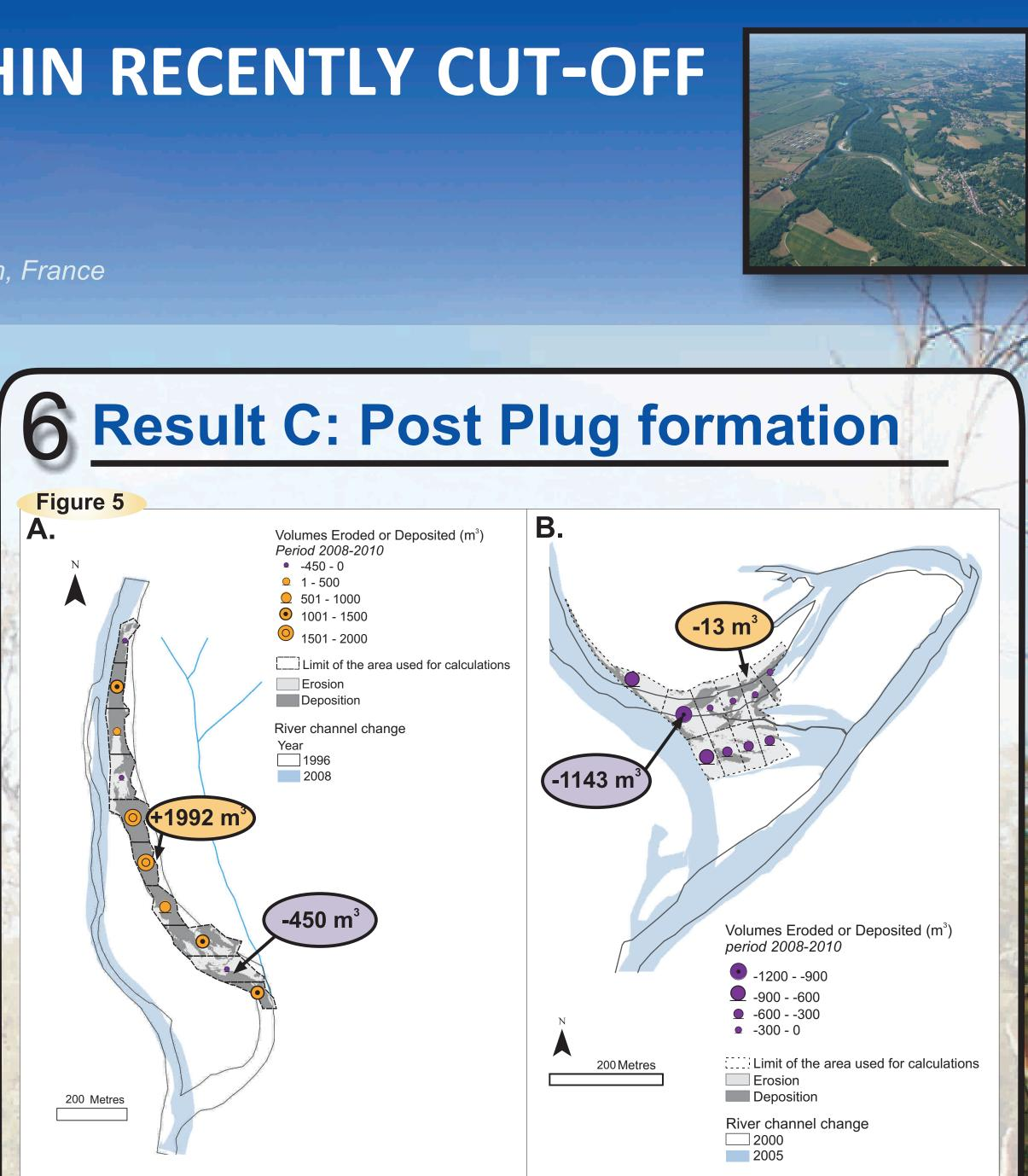
• Once the plug is fully developed upstream, direct bed-material transport is obstructed at the entrance of the former channel. Figure 5 shows a 2 year sediment budget (2008-2010) of the terrestrial part of the oxbows, indicating how the sediment plugs evolved after their formation.
