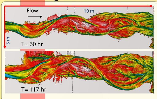
Meandering river forms in the experiment with cohesive floodplain-filling material
