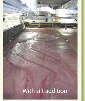
To test the effect of cohesive fines on channel pattern development, we conducted two parallel experiments. To one of the experiments we added a fine silt fraction (white silica flour) in the sediment feed in a ratio of 1:4. During Q<sub>high</sub> an extra amount of 0.5 L silt was added. The experiment ran for 120 hours.
