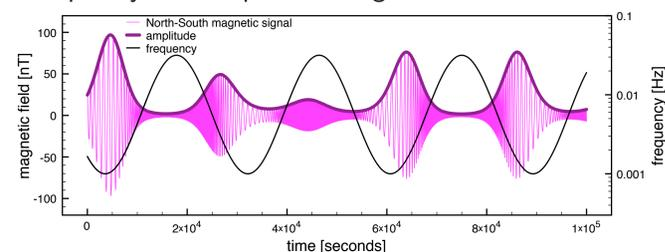
Figure 1: The magnetic source signal is defined by a chirp function with oscillating amplitude and frequency for statistical diversity.
