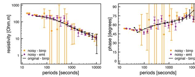
Figure 6: The noise level has been quadrupled compared to Fig. 4. Original data (black) is compared to (non) Fourier based methods.
