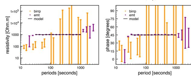
Figure 2: The Fourier Transform based BIRRP cannot analyse correctly the spectra for the non stationarity of the signal, unlike EMT.
