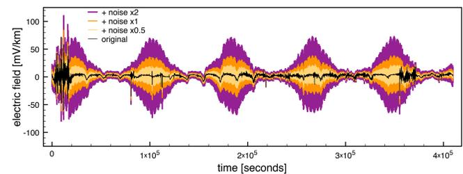
Figure 5: Non stationary noise is added to the electric fields of otherwise fair data to test its effect on different processing strategies.
