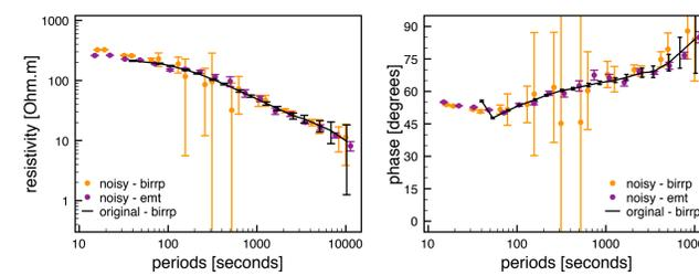
Figure 4: Fair real data is impaired by added non stationary noise. Original data (black) is compared to (non) Fourier based methods.
