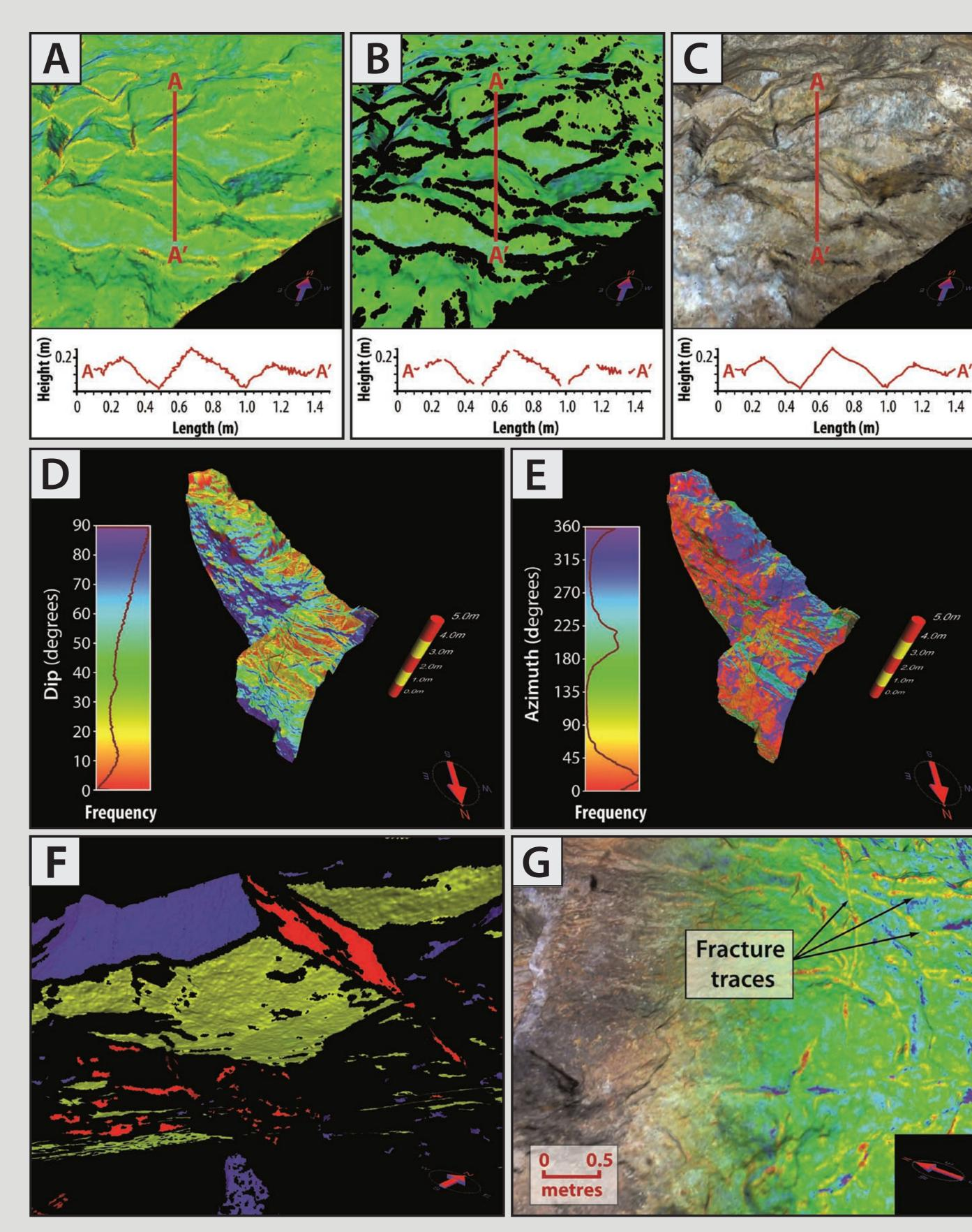
Fig 2. (A) The fidelity of TIN surfaces is limited by scanner ranging error (B). Regions of low coplanarity are filtered and smoothing operations conducted. (C) Surface is restored after smoothing operations. (D) Increases in frequency density for dip and (E) dip azimuth may indicate the presence of subparallel fracture sets. (F) Frequency distributions used to guide the filtering and extraction of fractures by sets. (G) Areas of low coplanarity indicate the presence of fracture traces.
