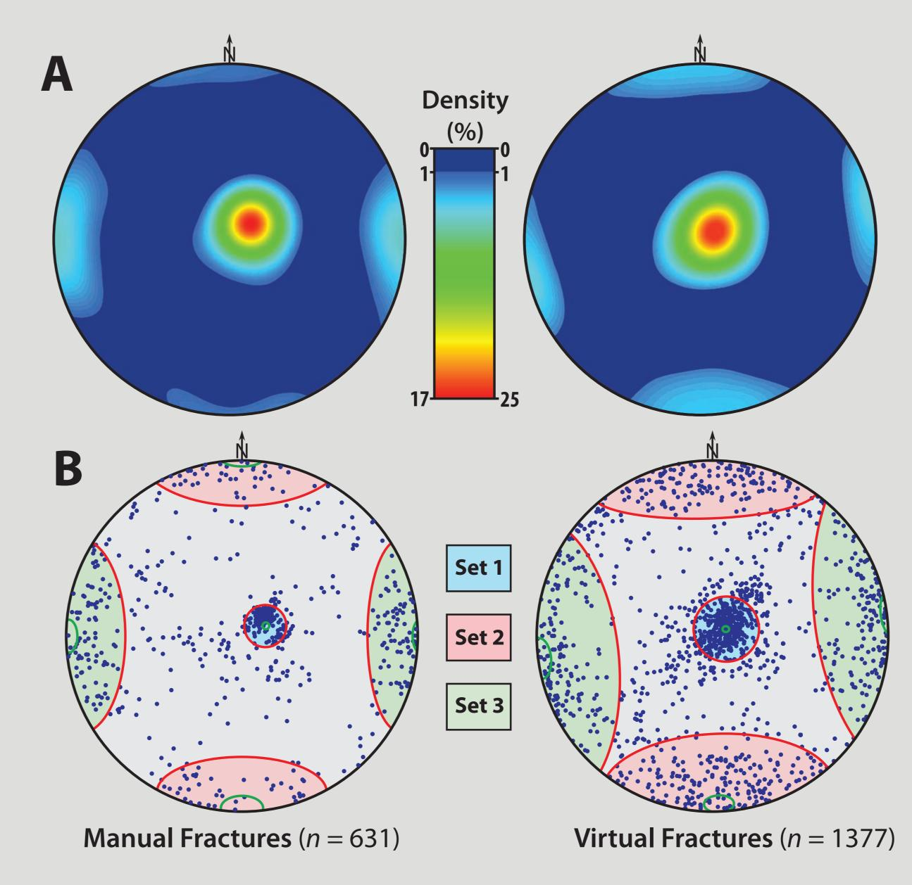
Fig 3. (A) Density plots showing manual scanline and lidar derived fracture orientation distributions. (B) NE-SW subhorizontal and north-south / east-west subvertical sets delineated using the clustering algorithm of Wallbrecher (1978).
