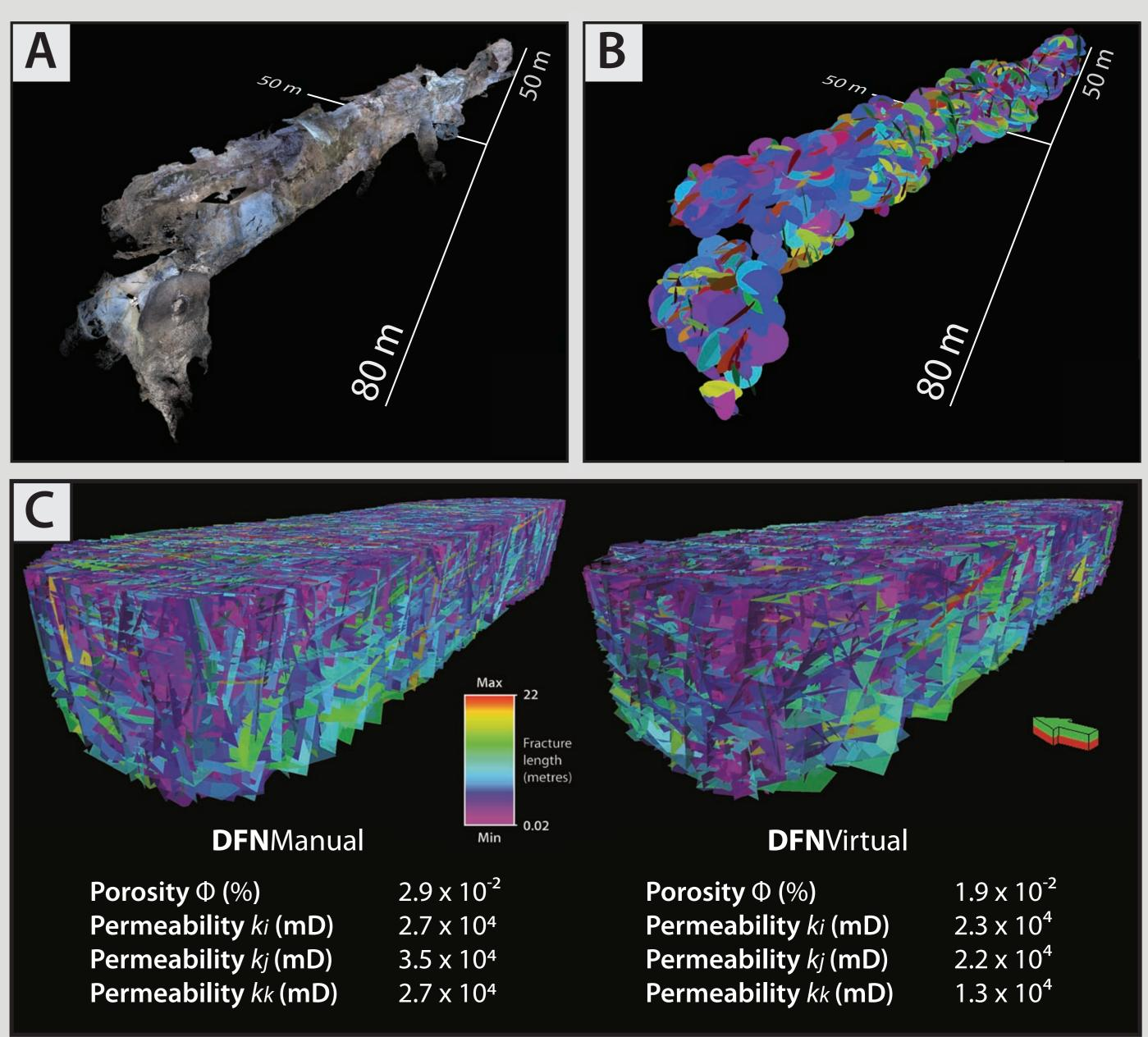
Fig 5. From outcrop model to DFN workflow summary: (A,B) Lidar outcrop models form the proprietory medium for the extraction of geometric fracture network properties. (C) Comparison of virtually and manually derived DFN models, with upscaled EPM properties indicated. Cumulative effects of spatial aliasing results in a 15-50% contraction in EPM properties in the lidar derived DFN.
