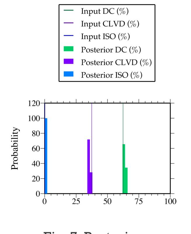
Fig. 7: Posterior distributions of the double couple (DC), compensated linear vector dipole (CLVD) and isotropic (ISO) components.
