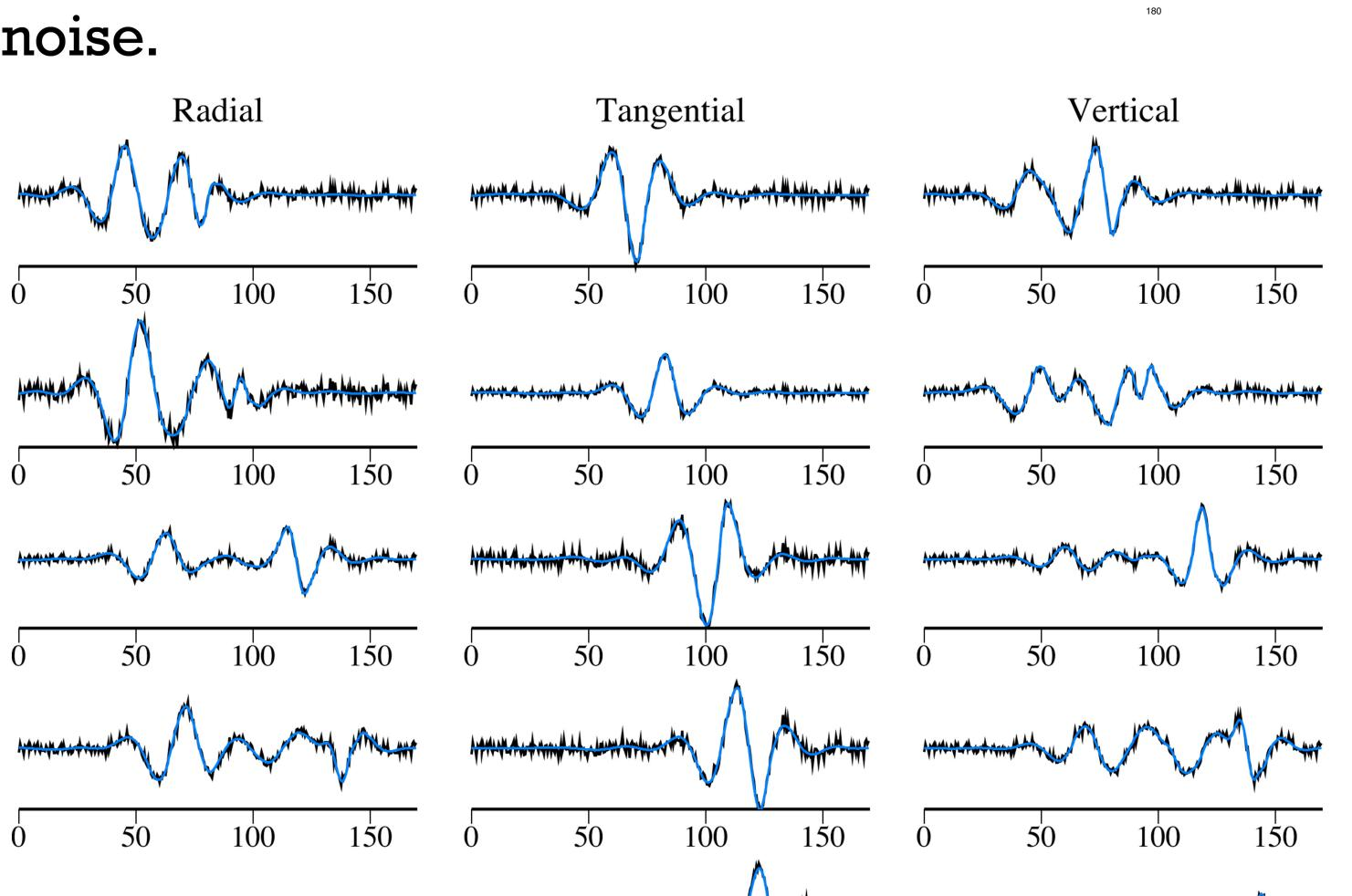
Fig. 1: Input synthetic seismograms with uncorrelated random noise (with a variance of 25% signal RMS) (black) and the best fit (minimum L2 misfit) solution (blue).
