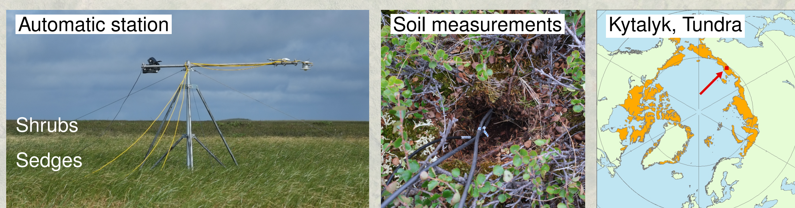
Fig. 1: Station for measuring radiative and soil heat fluxes, soil and air temperature (growing seasons 2013 and 2014); study site in the Arctic tundra (extent by Walker et al. (2005))
