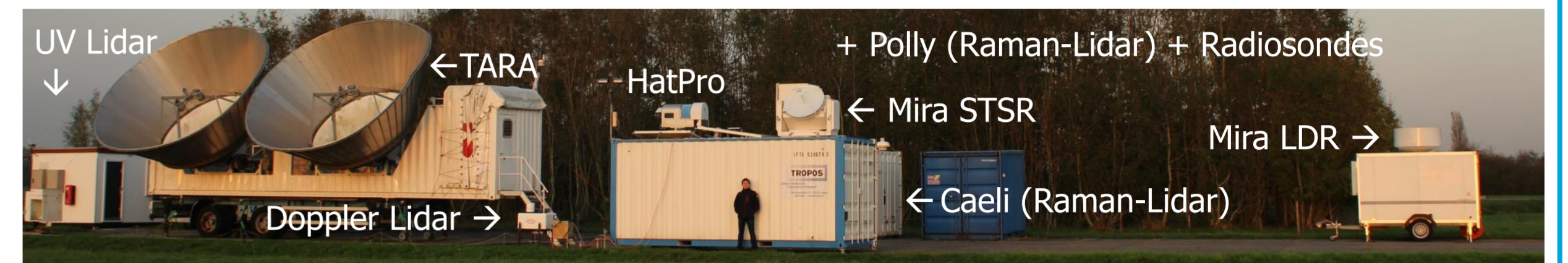
Shows the measurement setup of the ACCEPT campaign at the Cabauw experimental site for atmospheric research, Cabauw, the Netherlands.
