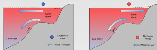
**Fig. 6:** Schematic of eastern boundary wind forcing and the respective changes in coastal sea level.
