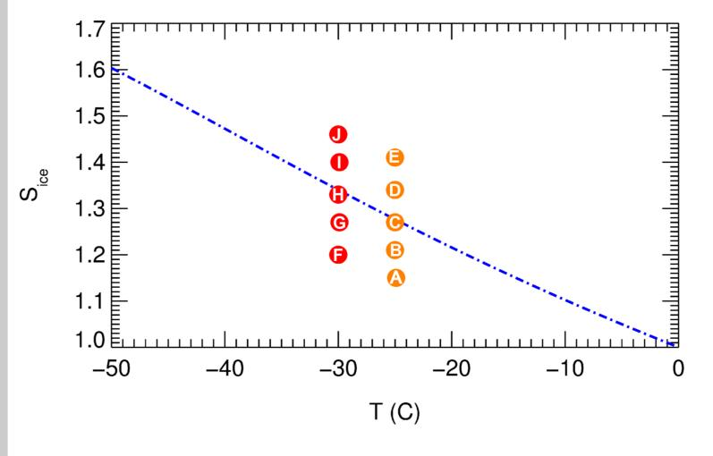
Calculated aerosol particle conditions during the stepwise scanning of an ice nucleation experiment with Saharan Desert Dust.
