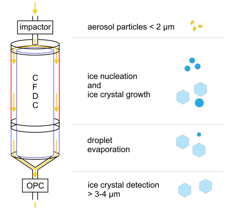
both walls ice-coated and at defined but different temperatures
