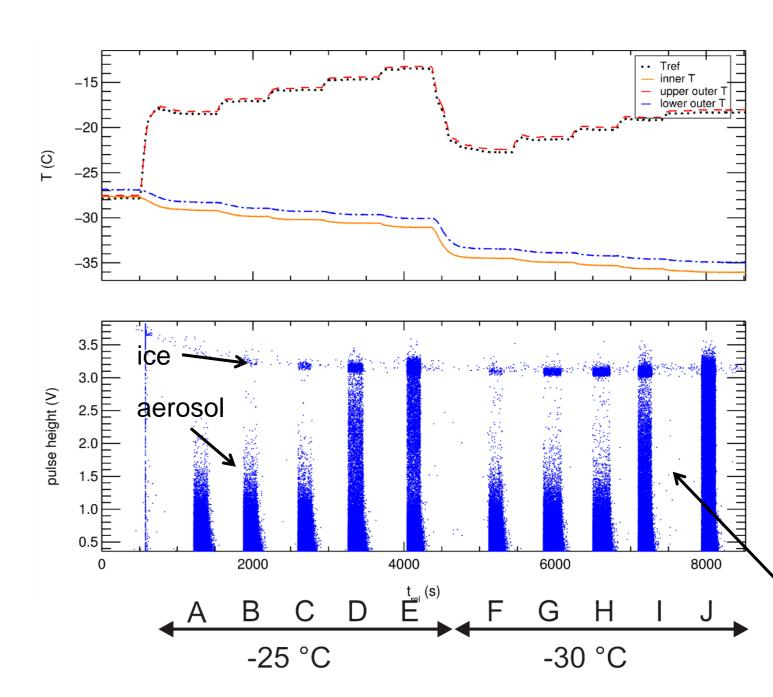
Wall temperatures together with the temperature of a reference sensor, which is located at the upper outer wall
