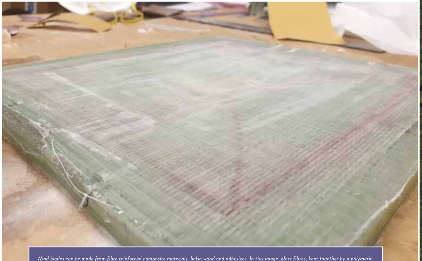
Wind blades can be made from fibre reinforced composite materials, balsa wood and adhesives. In this image, glass fibres, kept together by a polymeric 'glue,' are used for the most part in composites for wind blades.
