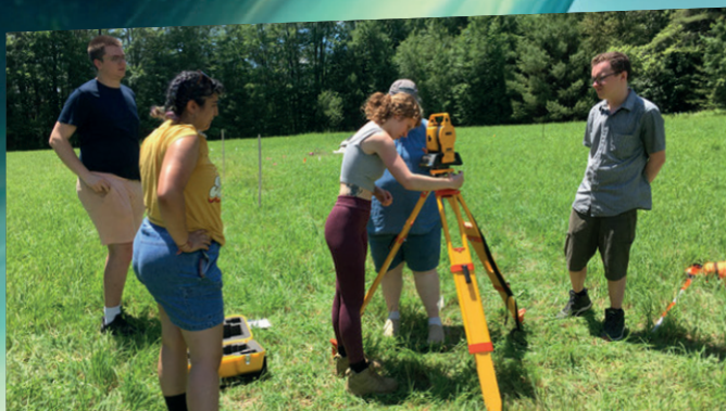
Emma shows fellow interns how to survey the mirror field using a total station.
