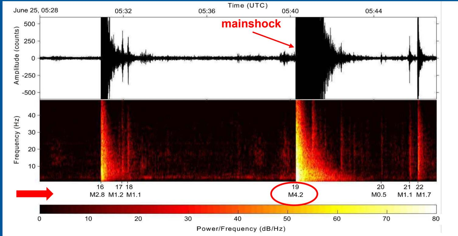
20 min data from the 290 m-deep 1 Hz vertical sensor at TESV indicates pre-shock seismicity including an M2.8 foreshock and at least four more events down to M0.5. The spectrogram indicates several more smaller events not seen in the waveforms.
