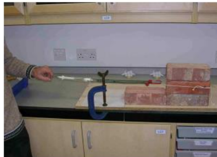
The brick 'earthquake' in action - b) Using a Newton meter to quantify the forces involved. The front brick is stopped from sliding by a board, held to the bench by a clamp. (Photos: P. Kennett)
