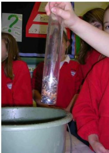
A jig being used to separate galena, barite, fluorite and calcite from a crushed sample
