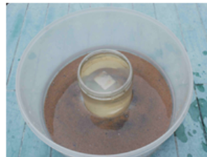
The 'continuous river bend' model set up with an even layer of sand and dense ore
