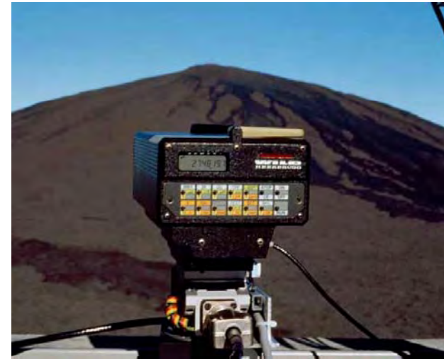
Automated geodimeter at Piton de la Fournaise volcano © P. Briole
