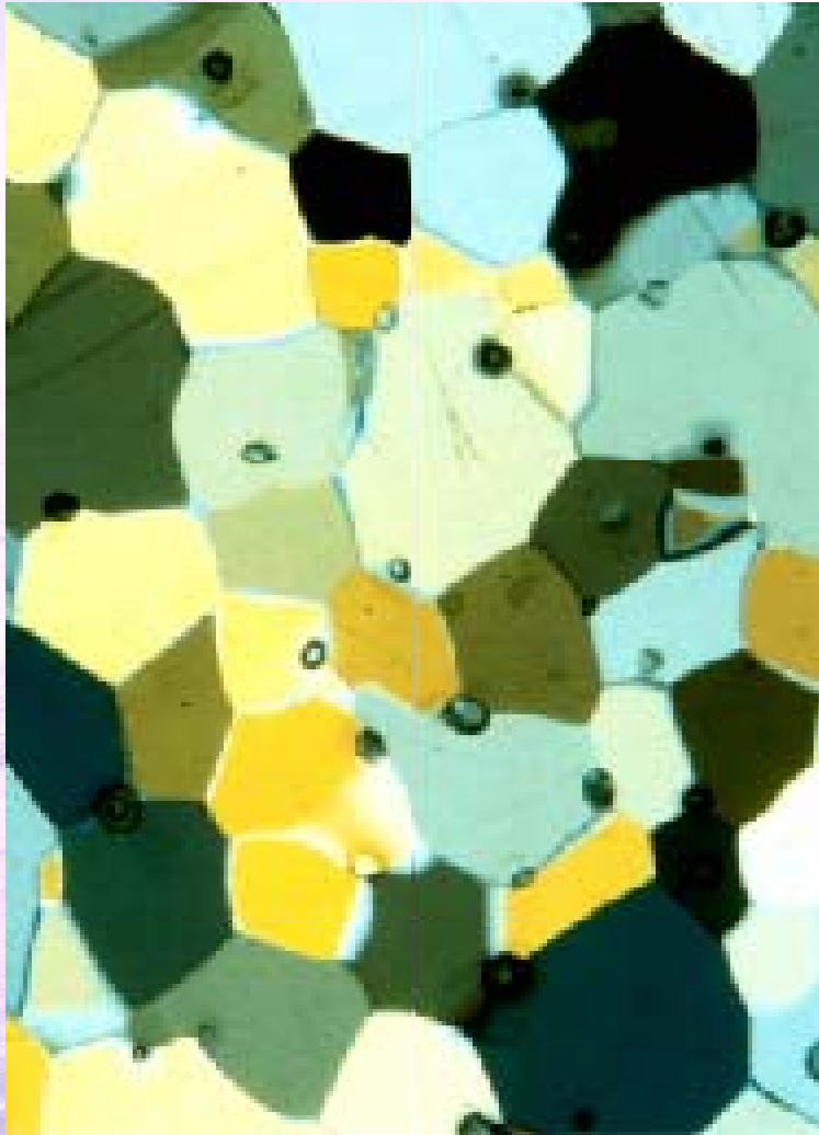
Natural ice through polarized light (sample size : ~2 x 3,5 cm) © V. Lipenkov, LGGE-CNRS
