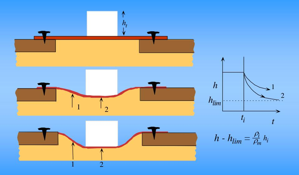
If ice melts, central load is decreased with time but meltwater also loads the membrane.
