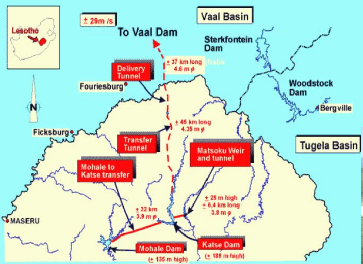
Phase 1 of Lesotho Highlands Water Project
