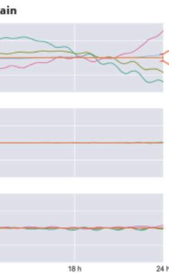
Fig 2a: Shows the difference between orbit iterations in the spatial domain. All integration methods have the largest errors in the along-track axis.
