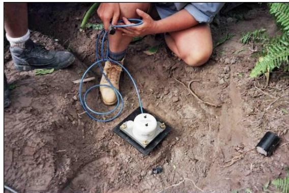
Tilt meter in use in Montserrat © University of Leeds
