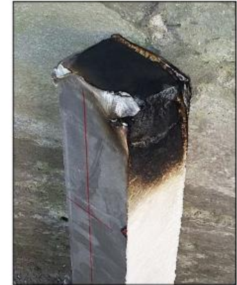
left - Polyisocyanurate board above - charred board
