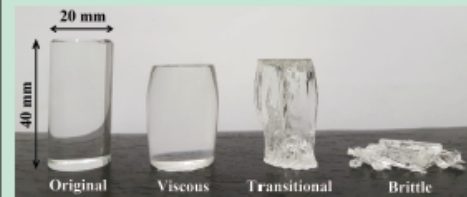
Figure 2: The original form of synthetic soda-lime-silica glass on the left and three samples recovered from the apparatus on the right, depicting three types of deformation (viscous, transitional and brittle).
