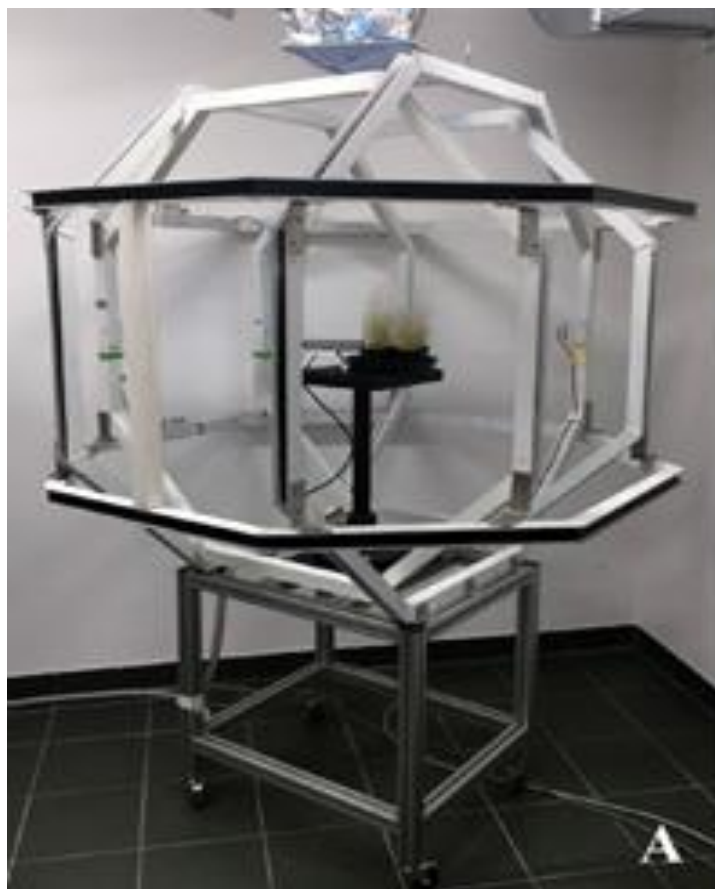
Triaxial Helmholtz coils systems (A) and power controls (B) At University of Turin (Italy)
