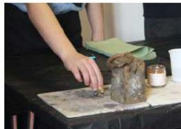
Step 4 – picking up iron crystals with a magnet, after crushing (Photos: Heidi Dobbs, RSC)
