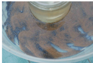
Ripple marks formed in the sand, with the dense ore trapped behind each ripple (All photographs by Peter Kennett)
